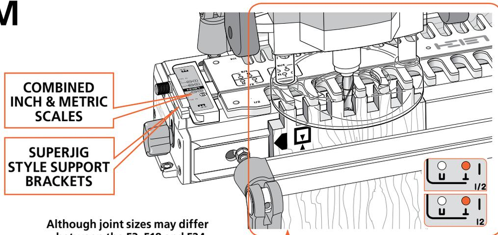
Although joint sizes may differ between the F3, F18 and F24, everything in these frames is operationally identical
