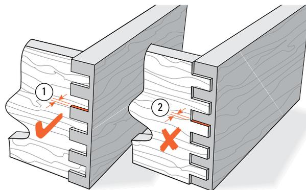
**7-6** The drawer front pins should project through the side sockets by no more than  $\frac{1}{64}$ " [0,25mm] for clean-up ①. If the sides project ②, adjust the template inward to suit.
