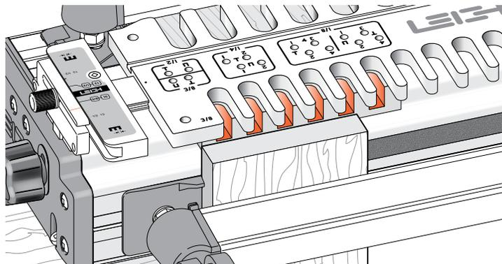
**7-5** Rout a test piece to test the scale setting for joint flushness and adjust the template in or out to produce the required flush fit.
