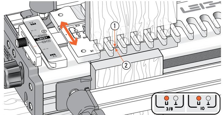
**7-4** Place one of the routed box sides vertically through the template with the rounded part of the fingers in the rounded guide crotches. Adjust the template so the front face of the side board ① is  $\frac{1}{16}$ " [1,5mm] in from the end edge of the box front ②. Lock the scales on the same setting at both ends.
