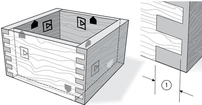
**7-1 Half-Blind Joints** Unlike normal box joints, the inside faces of half-blind box joint boards always face away from the jig body, and alternate edges are placed against the side stop. Set the depth of cut ① to about  $\frac{1}{8}$ " [3mm] less than the drawer-front thickness. Use only the "Symmetrical" board widths for half-blind joints.
