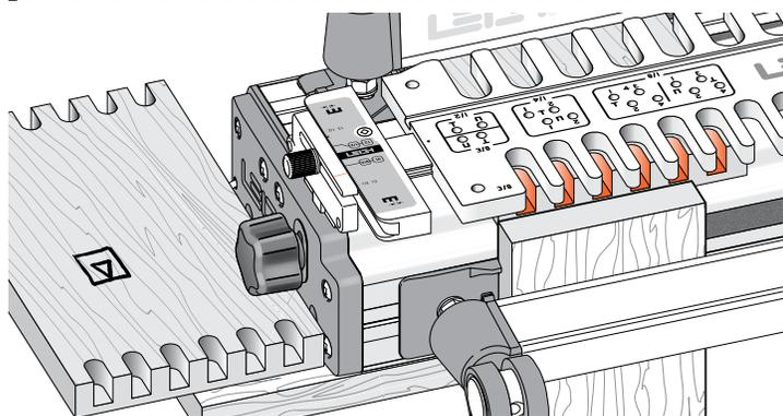
**7-7** When satisfied with the flushness fit, rout all the ends of the box fronts and backs in this mode.
