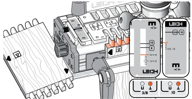
**7-2** Set the template pin on the **L** setting and the scales to the thickness of the box sides, e.g.  $\frac{3}{4}$ " [20mm] shown here. Rout the box side ends vertically in the front clamp.
