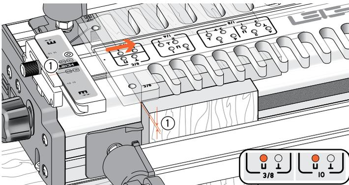
**7-3** Set the template pin on **U**. Clamp a scrap piece vertically in the jig front with its top end slightly above the jig body ①. Clamp a box front horizontally with the inside face **□** away from the jig body, and the front end edge against the scrap board.
