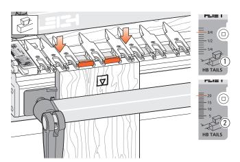
Where finger assembly scales overlay an illustration, the "inches" scale ① will be at the top, the "millimeters" scale ② will be at the bottom. Only the front "active" half of the scales are illustrated. For clarity, setting positions are indicated with a red line in the user guide only. On the jig, the lines are black.
