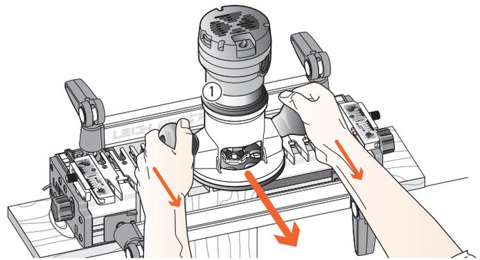
**5-6** If you insist on removing the router from the jig while it is still revolving, always pull it straight off the jig horizontally, and do not raise or lower the router until it is completely clear of the jig.
