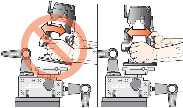
**5-5** Do not tilt the router on the jig. Keep the router flat on the jig assembly.
