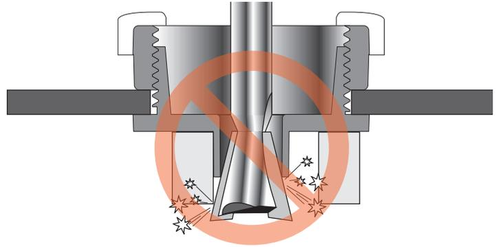
**5-8** Never release the router plunge mechanism when using dovetail bits. Check if your plunge router has a stop nut to prevent this from happening accidentally.
