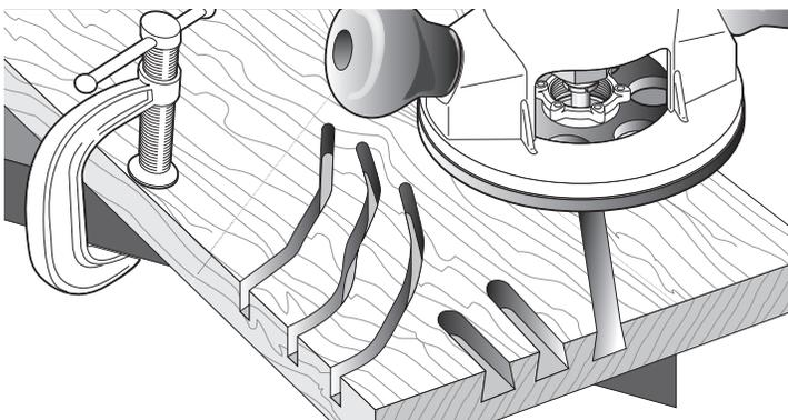
**5-9** If you have never used your router before, be sure to follow the router manufacturer's instructions for its use. Make plenty of simple open-face practice cuts *without a guidebush* before you try to use the router on the Leigh jig. You must, of course, always use a guidebush when routing on the Leigh Jig. ■
