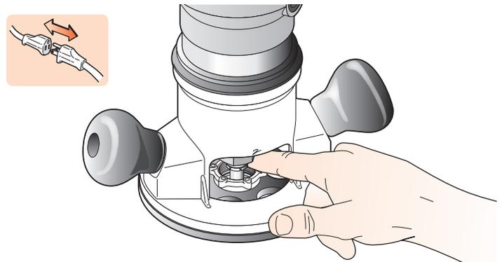
**5-4** Always disconnect the power source from the router when fitting bits or guidebushes, or making adjustments. Before connecting the router to the power source, make sure the bit and collet revolve freely in all the areas you plan to rout, and the bit does not touch the guidebush or jig.
