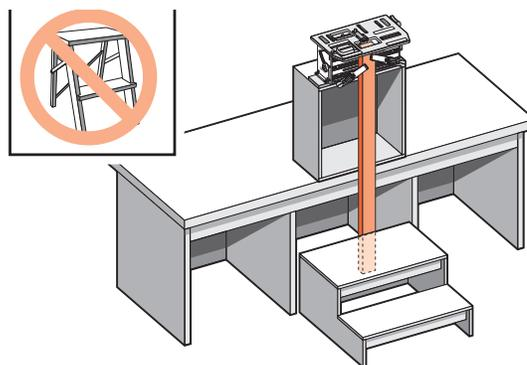
**6-18** To rout long vertical boards you could build a jig stand to mount on your bench. Make the stand/bench combination high enough to accept the desired board length. *Bolt securely to the bench.* Make a stable platform as shown here to stand on. **Don't use a folding step, these are unstable.** Other novel solutions: holes in (suspended) floor; jig bolted to deck or mezzanine railing; wall brackets. ■
