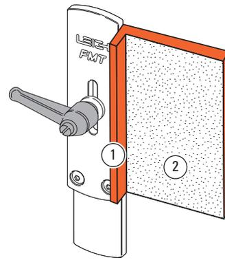
**6-4** This packing piece should include its own side-stop fence ① and if required frequently, should have sandpaper glued onto its outer surface for secure workpiece clamping ②. Sight and rout the tenons in the usual way with the packing piece in place. Then, remove the packing piece before sighting and routing the mortises. ■
