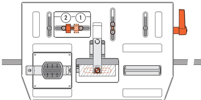
**6-7** Set the  $\frac{\circ}{\text{LR}}$  stops one at a time with the small block between the stops and post ①②. This ensures that the table movement is centered about the joint center-mark on the stock. Remove the block, but save it.
