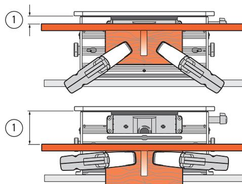
**6-20** Use the Leigh clamps to secure the bracket to the FMT Pro clamp face and adjust the distance below the table to slightly greater than the mortise piece thickness ①.
