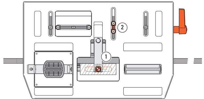
**6-6 Tenons** Mark the center as before. Position and sight the tenon ①, and lock the table. Set the  $\frac{\circ}{\text{FB}}$  stops against the post ②.
