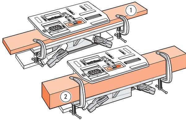
**6-21** Use C-clamps to hold the workpiece onto the bracket, with the workpiece rear edge touching the clamp plate. **Now raise the bracket so the workpiece touches the underside of the table.** Re-secure with the Leigh Clamps. The widest board in which a mortise may be centered is  $4\frac{5}{8}$ " [115mm] ①. The thickest capacity is 4" [100mm] ②.
