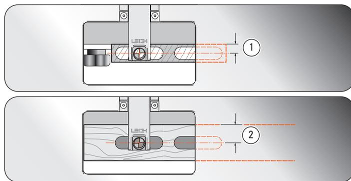
**6-2** Single or double (in-line) mortise and tenons are straight forward. Simply mount and sight and rout all the tenons as shown before ①, then mount and re-sight the mortises at the desired front-back position before routing ②.
