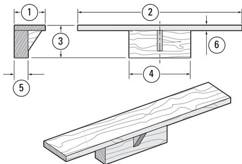
**6-19** Make this bracket to mount and mortise a wide board face, clamp pieces greater than Leigh Clamp 3" capacity, and center mortises on boards up to  $4\frac{5}{8}$ " [115mm] wide or even  $6\frac{3}{8}$ " [162mm].
