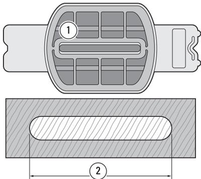
**6-5** The FMT Pro table movement allows for easy routing of odd-sized joints. For example, you may want to rout a 3" [75mm] joint ② and you only have a 2" [50mm] guide ①. Use this simple formula:
