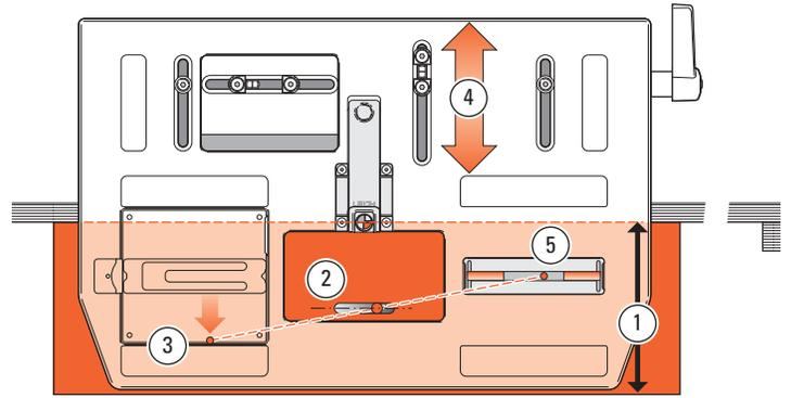
**6-22 Mortises in center of boards  $4\frac{5}{8}$ " to  $6\frac{1}{2}$ " [115 to 165mm]** ①: Mark mortise center on a test board ②. Using the guide recess front edge as mortise guide ③, adjust the table to center the mortise ④. Control mortise length with  $\frac{3}{16}$ " [5mm] dowel pieces in the pin track ⑤ (see 6-16). *Note: This is not a standard Leigh solution, but we thought it would solve this rare challenge.* ■
