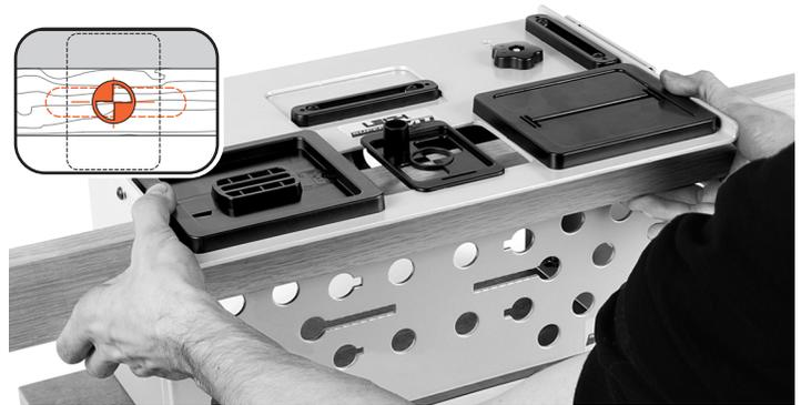
**4-16** Fit the sight and remove the sidestop fence if it is in the way. With the marked side of the mortise piece toward the clamp plate, either move the board left and right to align the cross with the sight and clamp in place, or clamp in place first and move the table to align the sight. Remember, you previously set the **FB** limit stops to allow only left/right movement.
