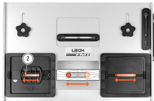
**3-25** Mortises are routed with the guide pin running in the inside mortise slot of the guide ②. Always route the mortise slightly deeper than the tenon length. **Note: In most constructions, only one tenon and perhaps two mortises need to be cross marked and sighted. Please read all of the procedural chapters to gain the utmost efficiency from your Super FMT. ■**
