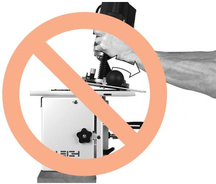
**3-32** Do not tilt the router on the jig.
