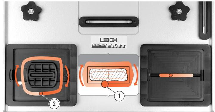
**4-12** Read 4-12 through 4-14 before routing. With guide pin in near side of guide recess, switch on router power and with firm control, move it in until the bit lightly touches the tenon workpiece. **Very carefully, with the bit very lightly engaging the wood surface, “climb rout” clockwise around the tenon piece ①.** Maintain very light bit contact. **Do not run guide pin on guide yet ②.**
