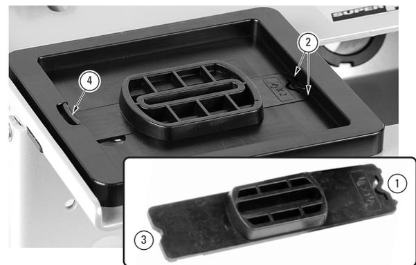
**3-16** Two small projections on the Guide ① fit into undercuts on the right side of the guide recess ②. The left end of the Guide ③ is pushed down and retained by the spring-loaded Guide Latch ④.
