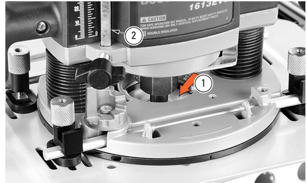
**3-31** Make sure the router collet does not contact the Super FMT sub-base at full plunge cuts ①. Set the router plunge stop rod as necessary to prevent this ②.
