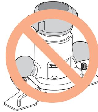
**3-35** The Super FMT must only be used with a plunge router. Never, ever use a fixed base router!
