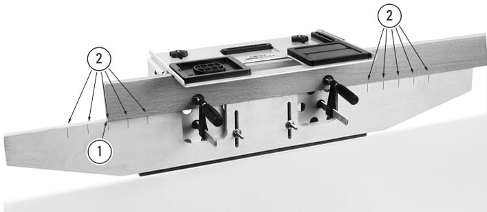
**4-31** Multiple mortises in “ladder” type construction are rapidly routed. Mark all mortises on only one piece (only one of the marks needs a front-to-back mark!). Sight the first mortise (cross) to set the table and mark the top of one outrigger in line with workpiece end ①. Table locked, move workpiece, sighting each successive mortise line, marking the outrigger(s) ②. To rout, align unmarked board ends with outrigger marks ②. ■
