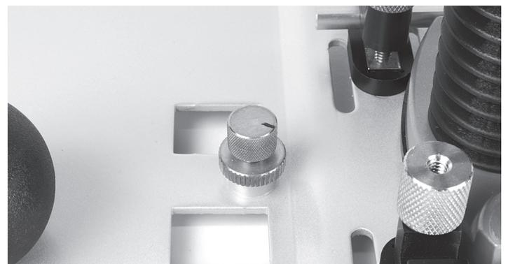
**4-26** Once you've established the guide pin setting for a specific bit/guide combination, record the setting on the following page. For example:  $\frac{5}{16}'' \times 1\frac{1}{2}'' [8 \times 35\text{mm}]$  "up  $1\frac{3}{4}$  turns". Using the same bit and guide next time, use the recorded setting for a good fit first time. Note: Different wood species may require slightly different settings. ■
