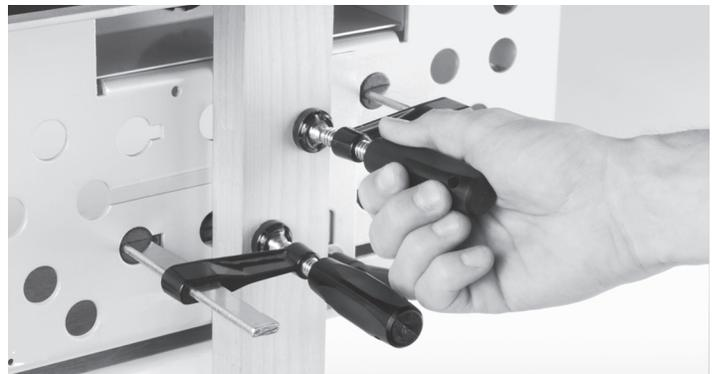
**3-4** ⚠ **Do not over tighten the clamps;** excessive force may damage the workpiece. A few minutes of trial and error testing will soon give you the feel for the correct clamp tension.
