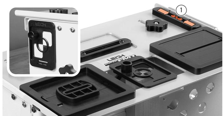
**4-6** Unlock the two  $\text{FB}$  front/back limit stops. Move both so they touch the Stop Post, and tighten both stops ①. This prevents front-to-back movement of the table when later sighting the mortise. Remove the sight and store it at the end of the jig.
