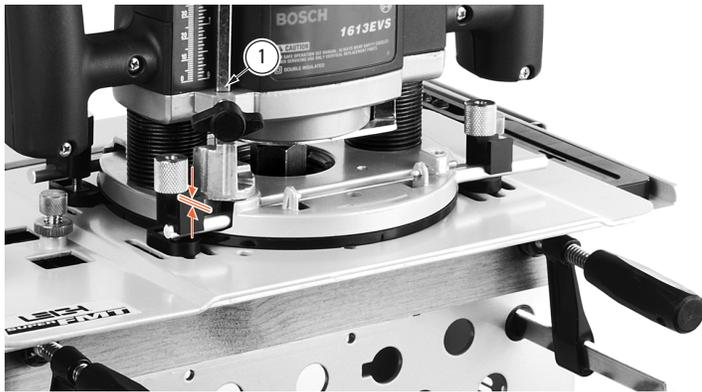
**4-17** Remove the sight and place the router/sub-base assembly on the jig, the left hand guide pin in the mortise slot part of the guide. Now raise the plunge stop rod ① slightly, say  $\frac{1}{32}$ - $\frac{1}{16}$ " [1-1,5mm] to allow the mortise to be routed slightly deeper than the tenon to ensure perfect tenon shoulder flushness on the finished joint.
