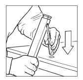
Take the clamp knobs and tubes off the jig. Put the Leigh finger adjustor screwdriver through each tube's large bolt hole and into the end plug. Strike down sharply against a solid surface to remove the old plug.
