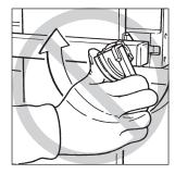
**3** Do not use the lever as a torque arm. Adjust the clamp tension only with the clamp disengaged.
