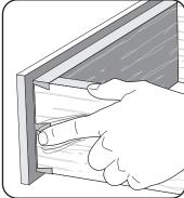
**12-8** Make sure you select a dovetail bit that has a working depth of cut less than the rabbet height ①. Otherwise, you will rout into the rabbet lip ②.
