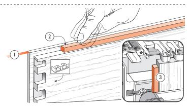
**12-6** If the lip thickness ① is greater than  $\frac{3}{8}$ " [9,5mm], it will not fit under the side stop. Block the drawer side away from the front side stop by exactly rabbet depth (*see 12-3*). Make up a block ② and stick it to the jig face ③ with double-sided tape. Make sure it touches the side stop. This will offset the drawer side from the side stop by the width of the rabbet, and align the sockets with the pins.
