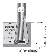
IMPORTANT: Add ~1/8" [3mm] to the depth of cut for pin board thickness NOTE: See 10-35 chart on p.38 for range of tail board thickness NOTE: Bits 80-8 and 120-8 are included with the jig
