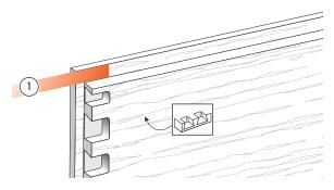
**12-7** If the rabbet width ① is greater than  $\frac{3}{8}$ "[9,5mm], the drawer side must be offset from the front side stop by the depth of the rabbet minus  $\frac{3}{8}$ "[9,5mm]. Make up a block to this measurement and stick it to the face of the jig, touching the front side stop. This will offset the drawer side away from the side stop and align the sockets with the pins.
