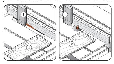
**12-5** An easy accurate way to do this is to rabbet the end of a scrap piece ① vertically over a dado blade or router bit at the same time as you rabbet the drawer front (horizontally) ②.
