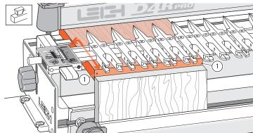
**11-10** Place a sample drawer front from  $\frac{5}{8}$ " to  $\frac{1}{2}$ " thickness [16 to 38mm] in the rear clamp. Clamp with the side edge against the left rear side stop, front end edge touching flush across the rear of the front board ①. Note: the  $\frac{5}{8}$ " [16mm] minimum thickness can be reduced if using other shallower bit depths. ! *Board edges must be square.*
