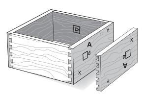
**11-24** Assemble the drawer. As with through dovetails, it doesn't matter which edge of any of the boards are at the top or bottom, the drawer will still fit together e.g. pin board "A" can be up either way.
