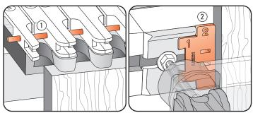
**11-7 Stop Rod and Dovetail Spacer** The stop rod is inserted in the fingers ① to convert them from deep tail sockets to a shallow fixed comb. The flexible stop rod is fed through the holes in the fingers from the "far" end of the jig. The **Dovetail Spacer** (note the dovetail shaped notch) snaps into the channel against the left-hand front side stop ② to correctly offset the drawer sides from the drawer fronts. After setup, the Spacer stays in place for the complete procedure.
