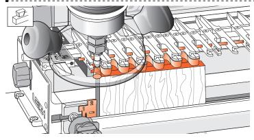
**11-17** Now rout in and out from left to right. Follow the guides in on the left of each finger opening to touch the stop rod and come out on the right. The pins, tails and sockets are formed simultaneously.
