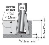
IMPORTANT: Add ~1/s" (3mm) to the depth of cut for pin board thickness NOTE: See fig. 11-9 on p.42 for range of tail board thickness NOTE: Bits 120-8 and 80-8 are included with the jig
