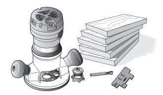
**11-5 Routing a Test Joint** You need a router, the e7-Bush set at No.10 (see chapter 3 for e-Bush instructions) and the 80-8 ½"[12,7mm] 8° dovetail bit. *Note:* The No.80-8 bit routs at a shallower ~½"[13mm] depth on single pass dovetails than on regular variably spaced joints. For this test, start with the No.80-8 bit projecting ½"6"[24mm] from the router base.
