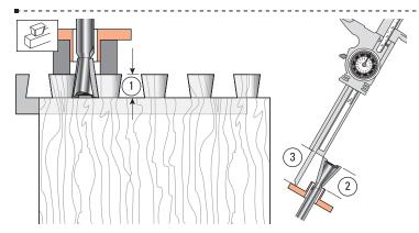
**11-19** Keep the test tail board that fits well, and mark it with the number of the bit you used to rout it. For quick set-up next time, clamp this tail board in the jig as a *depth-of-cut gauge* ① to show how far to lower the bit. Better yet, measure the bit projection from the end of the guidebush ② or guidebush flange ③ and record this for fast set-ups in future.
