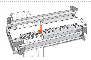
**11-6** This is a typical fixed template comb type jig. The comb depth ① is usually dimensioned to suit the most popular drawer side thickness of  $\frac{1}{2}$  [12,7mm].
