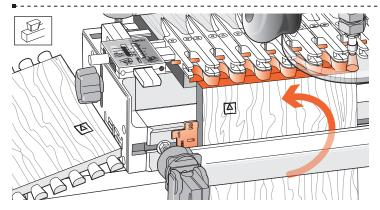
**11-23** To make a box, repeat the procedure four times, ensuring the drawer fronts, rears and sides are all rotated correctly in the jig, keeping the inside face  $\square$  of the boards away from the jig.
