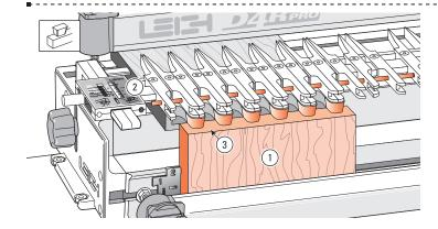
**11-25** For tail (drawer side) boards thicker than 9/16" [14,29mm] ①, set the scale to 1/2" [12,7mm] ② and leave the stop rod in place. **Do not** set the scale to the actual tail board thickness. With thicker boards, more of the inside portion of the tail board ③ will be routed away. Slight scale adjustments may be required for a flush fit. See figures 11-20 through 11-22.
