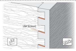
**11-20** When you have the proper tightness of fit, check the flushness. The tails should be under flush to the pins by *no more than* 1/64"[0,3mm] to allow for cleanup (exaggerated here). Any concentricity errors in the collet and guidebush on different routers will affect this tolerance.
