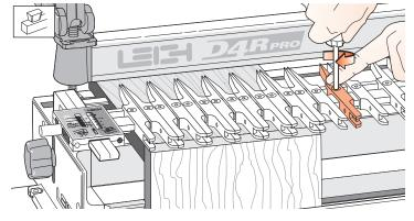
**11-14** Move any spare fingers so that they will support the router and **tighten all loose fingers**.
