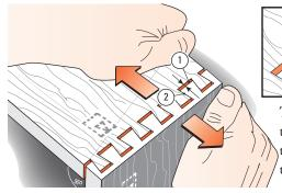
Test the joint fit. Pull the joint apart so the tails are tight against the socket sides (2)
