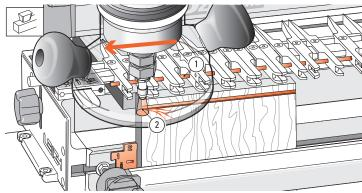
11-16 Insert the Stop Rod through the holes in the fingers ①. For the first light cut move the router from right to left. Make sure you control it firmly, because it is driven in this direction by the bit. Only the tip of the bit should be cutting on the first cut ②. This back, or climb routing, leaves a very clean shoulder when routing side grain.
